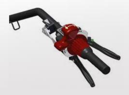
For both forwarding controls, a notch sector allows the operator to easily and repeatedly fix the position of the lever or of the knob. A central area without notches lets the lever or the knob to be positioned as desired, so that the machine can operate at a very slow speed.
